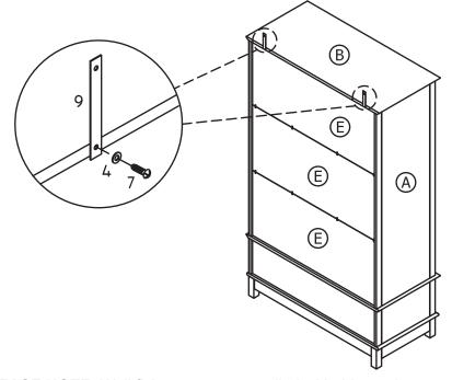
WARNING: In order to prevent overturning, this product must be used with the wall attachment device provided.
