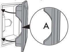
7. Press the cover completely down so that it attaches perfectly to the bulb support.
