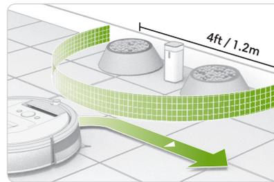
**Halo Mode:** When the switch is in the “down” position (↓), the device creates a protective zone that the Roomba will not enter. This prevents the Roomba from bumping into items you want to protect (e.g. a dog bowl or vase) or crossing into undesired areas (e.g. a corner or under a desk). The Halo is invisible and reaches approximately 24 inches (60 centimetres) from the centre of the device.
