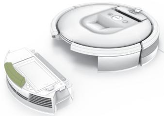
1 Press bin release button to remove the bin.
