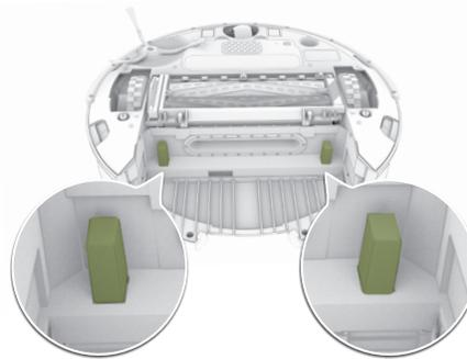
3 Wipe the inner and outer sensor ports on the bin with a clean, dry cloth.
