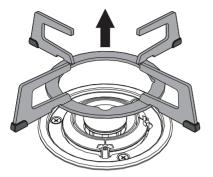
2. Remove the flame-spreader crowns and relative burner caps.
