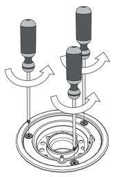
5. Remove the screws that fasten the hob top to the burner casing (the figure shows the 60 cm model as an example).
