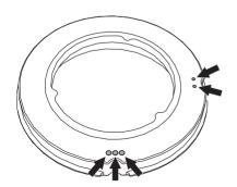
Refit the flame-spreader crowns making sure that they are correctly positioned in their housings with their respective burner caps.
