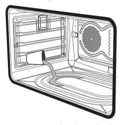
Spray a water and washing up liquid solution inside the oven using a spray nozzle. Direct the spray against the side walls, upwards, downwards and towards the deflector.
