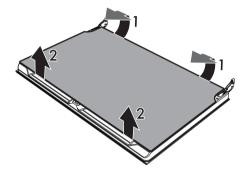
Some models have an intermediate glass pane. Remove the intermediate glass pane by lifting it upwards.
