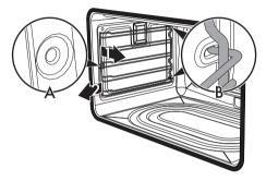
When cleaning is complete, repeat the above procedures to put the rack/tray support frames back in.
