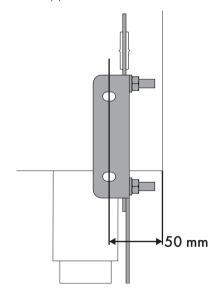
7. Move the bracket onto the wall and mark the position of the holes to be drilled in the wall.
