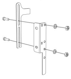
4. Align the base of the hook on the fastening bracket with the base of the slot on the wall fastening plate.
