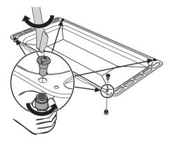
2. Position the rotisserie supports in the bushings as shown in the figure below.
