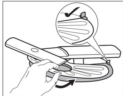
7. Reassemble the filters (B) and (C).
