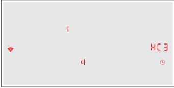
3. Set the  $\overline{\mathcal{Q}}$  value on the control panel. WLAN is deactivated and the  $\widehat{\mbox{\bf r}}$  symbol on the control panel goes out.
