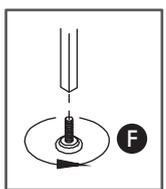
**Note:** Once the Supporting Legs are secured in place, unscrew the Adjuster slightly, ensuring there is a 5mm gap between the Adjuster and hard point of the floor.
