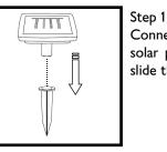
Connect the solar panel to the spike "B". To avoid damaging the solar panel, install the ground spike into soft ground and then slide the solar panel onto the spike.
