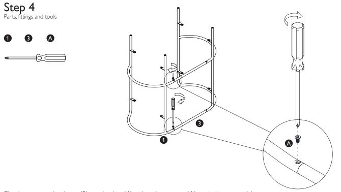
Fix the connecting bars (3) to the leg (1) using the screw (A) and the screwdriver.
