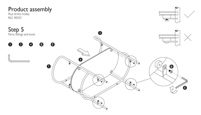
With 2 people carefully lay the trolley on its back on a soft surface. Support the glass (4) and align with the brackets located on the frame. Insert the allen bolts (B) with the allen key (E). Do not fully tighten at this stage until the trolley has been placed on its wheels to ensure the item is level.
