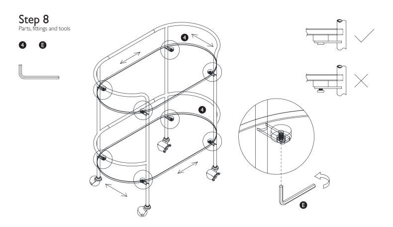
With 2 people carefully place the trolley onto its wheels. With the allen key (E) firmly tighten all the allen bolts.
