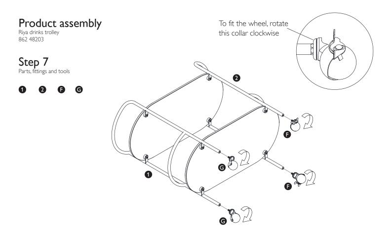
Locate the wheels (G,F) onto the legs (1,2) as shown above. To fit, turn the collar clockwise as shown in the detail.
