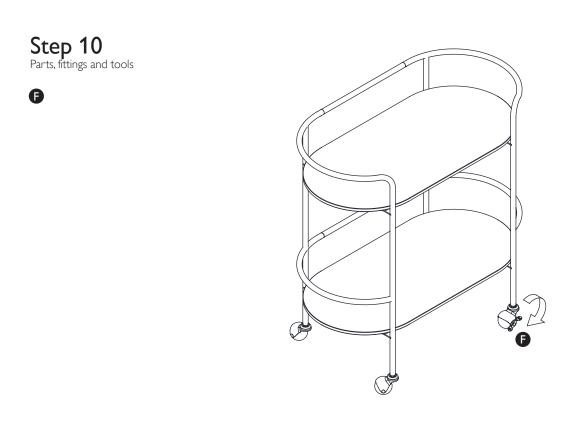
For security two wheels are fitted with locks. Please ensure the wheels are locked when the trolley is stationary.
