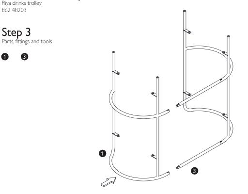
Locate the leg (1) onto the connecting bars (3) as shown above.
