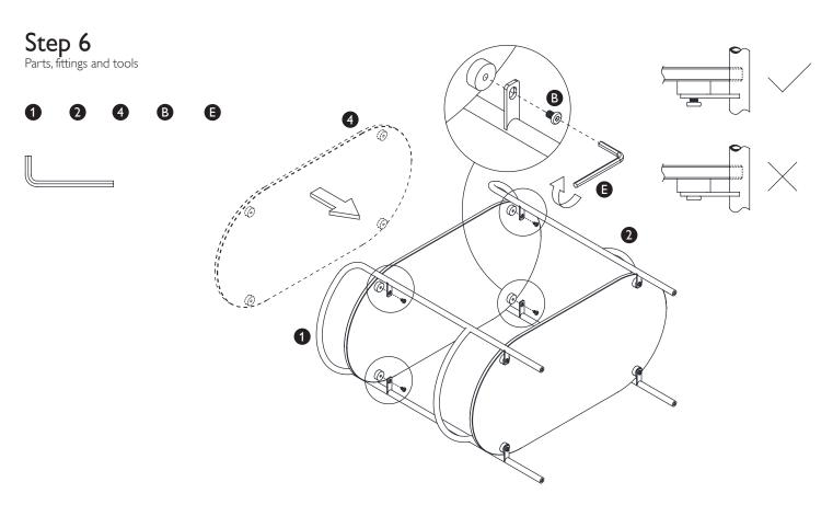
With 2 people carefully support the glass (4) and align with the brackets located on the frame. Insert the allen bolts (B) with the allen key (E). Do not fully tighten at this stage until the trolley has been placed on its wheels to ensure the item is level.
