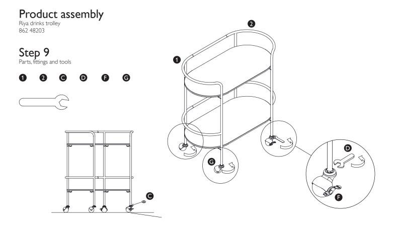
Using the open end spanner (D) firmly tighten the wheel nuts as shown in the detail above. Should the trolley require a small amount of levelling remove the necessary wheel and install a washer (C). Refit the wheel and tighten securely.
