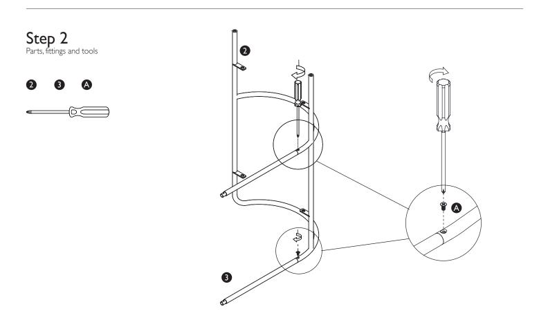
Fix the connecting bars (3) to the leg (2) using the screw (A) and the screwdriver.
