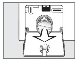
■ Remove the drain filter completely.
