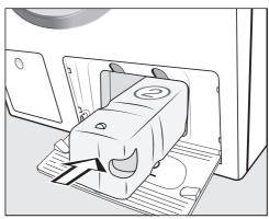
■ Push the **UltraPhase 2** detergent cartridge into **compartment 2** until it locks into position.
