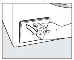
■ Open the drain pump access panel.
