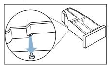
Turn the condensation container 180° again and insert the stopper into the recess in the top of the condensation container.
