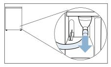
**Note:** The appliance comes delivered with the condensation hose already fitted to the socket.
