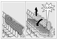
\* Depending on the model, a 3-fold height adjustment is possible. To do this, first place the etagere vertically and pull up, then place at a slight angle, push down to the required height (1, 2, or 3) and snap into place.
