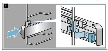
Keep the "PUSH" tab pushed back and swing the rail out (fig. 2).
