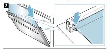
Slide the outer panel back in and make sure that it is sitting correctly at the bottom in the retainer (fig. 4).
