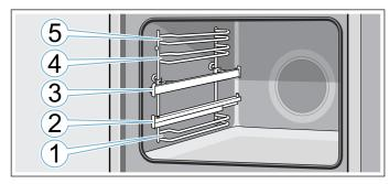
Always insert accessories between the two guide rods for the shelf position.
