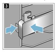
4. Release the "PUSH" tab; the retainer will hook into place (fig. 4). Then pull the rail out as far as it will go and slide it back in.
