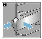
Pull the rail out towards you until the retainer at the back unhooks (fig. 3).
