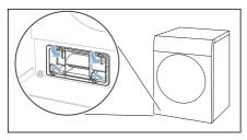
**4.** Pull the heat exchanger cover out by its grip.
