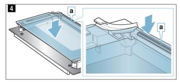
Slide the outer panel back in and make sure that it is sitting correctly at the bottom in the retainer (fig. 5).
