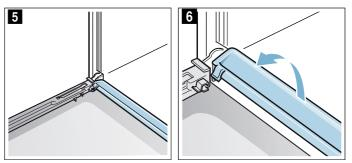
Clean the panels with glass cleaner and a soft cloth. Wipe the condensate trough with a cloth and some hot soapy water.
