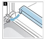
Slide each inner panel back in and make sure that it is sitting correctly at the bottom in the retainer (fig. 2).
