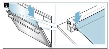
Slide the outer panel back in and make sure that it is sitting correctly at the bottom in the retainer (fig. 4).
