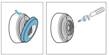
2. Open the closure of the temperature sensor. Remove the battery from the lower section of the housing and insert a new battery (pay attention to the correct orientation of the battery poles).
