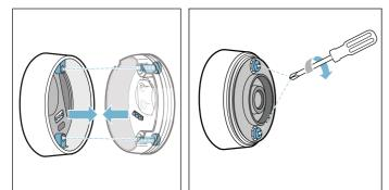
4. Reattach the silicone cover to the lower section of the temperature sensor housing.
