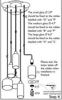
Ensure the house electricity supply is switched off at the fuse board.
