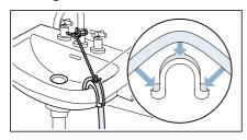
Drainage into a siphon The connection point must be secured using a hose clamp with a diameter of 24 - 40 mm (available
