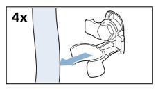
2. Unscrew and remove all four transport brace screws.
