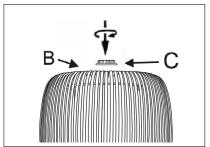
Step 1 Tighten the plastic washer (C) to fix the lampshade (B).
