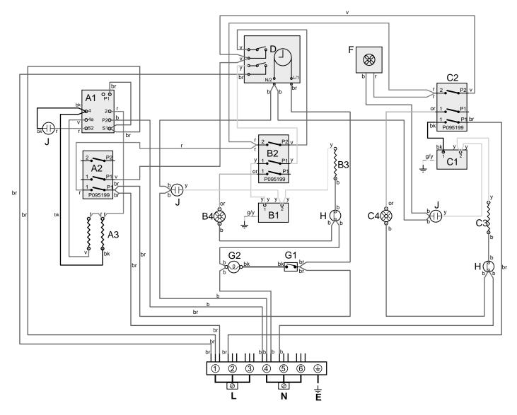
**Key**The connections shown in the circuit diagram are for single-phase. The ratings are for 230 V 50 Hz.
