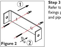
Refer to Figure 2. Attach the fixing bracket to the wall using the fixings provided. Take care to avoid damaging any concealed wiring and pipes.
