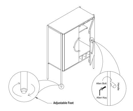
Place the Product upside down and place the handle.(2) on the matching holes. Tighten with Allen bolt with the help of Allen Key. Repeat the same procedure for second handle
