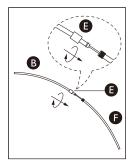
3. Insert tube (F) into tube (B) and turn part (E) until tight to secure tube (F) to tube (B).
