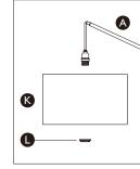
7. Socket ring (L) comes pre-assembled to the socket. In order to attach shade (K), unscrew socket ring (L). Then, place shade (K) onto the socket and screw back on socket ring (L) to secure shade (K).
