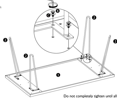
Do not completely tighten until all bolts are inserted and the legs are in the correct angle.
