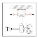
Excess cable must be carefully located inside the ceiling cup or within the ceiling cavity itself. Carefully offer fitting (D) over mounting bracket then secure in place with the screws and any washers removed earlier. Take care not to damage the wiring.
