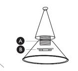
To attach the glass shade remove shade ring (B) from threaded body (A), place glass shade over threaded body (A) and replace the shade ring (B), tighten with light pressure.
