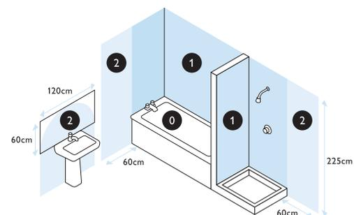
Installation in a bathroom. This product has special protection against the ingress of moisture and is IP44 rated. It is suitable for use in Zone 2 and outside zones of a bathroom. If installing in a bathroom, a 30mA RCD must be used in accordance with IEE wiring and the Building regulations.
