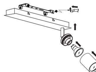
Re-attach the product to the fixing bracket and tighten the side screws. Take care not to trap any wiring. Fit the bulbs. Simply unscrew the head to access the lampholder. Once the bulb has been installed, refit the head, ensuring the sealing ring is in position and tighten to secure. Replace fuse or circuit breaker and switch on. Your light is now ready for use.
