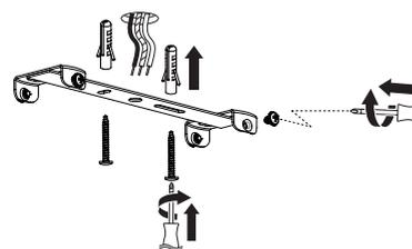
Remove the fixing bracket from the ceiling cover and attach to the ceiling using the screws provided. Ensure there is a joist at the point of fixing to support the weight of the product. Take care to avoid damaging any concealed wiring and pipes.
