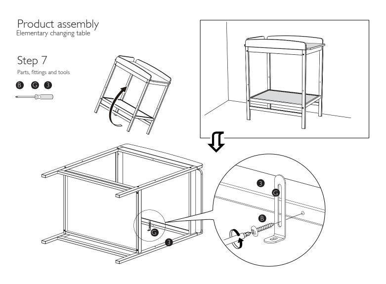
The Metal "L" Bracket (G) can be installed on part 4( Crossbar) or part 3 ( L/R side panel)
