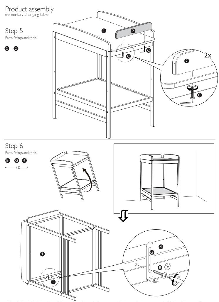
The Metal "L" Bracket (G) can be installed on part 4( Crossbar) or part 3 ( L/R side panel)
