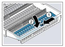
2. To fold down the front prongs, push the lever forwards and fold down the prongs ①.
