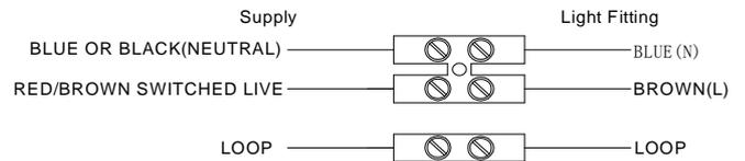
Check all wires are tight in the terminal block, and no loose strands are left out. Cover with insulating tape.
