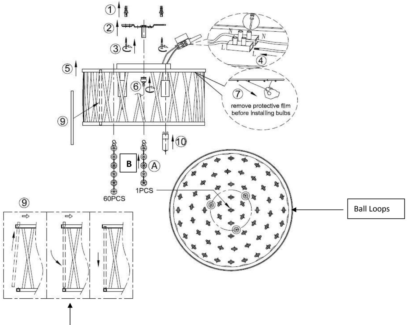
Slide chrome rods through the hole in the top frame from underneath and once in place the rods will locate on the bottom frame as per drawing
