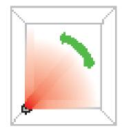
To start the appliance oscillating, press the oscillation control button. To stop the appliance oscillating, press it again. The appliance will not
