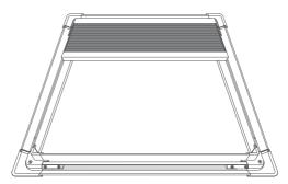
Loosen the screw then pull through the cord to adjust the tension. Pull the excess cord through by 5-10mm further to increase the tension or the opposite direction to loosen.
