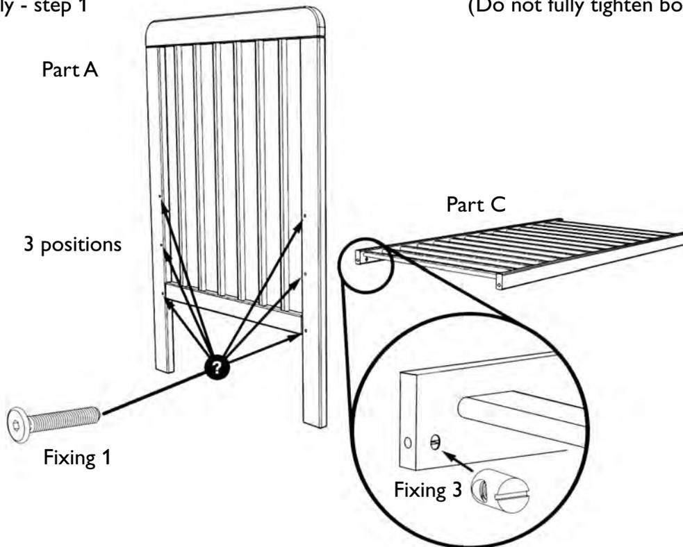
Push two barrel nuts (fixing 3) into the holes at one end of the base (part C) as shown above. Make sure that the slots are visible and, if necessary, use a flat-headed screwdriver to ensure that the slots point towards the holes in the ends as shown. Select one of the 3 base heights and attach an end (part A) using two 65mm bolts (fixing 1). Do not fully tighten the bolts at this stage.
