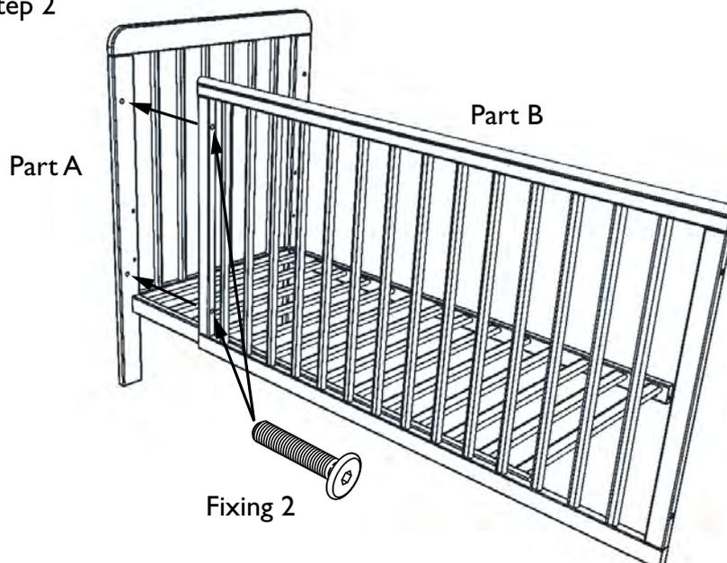
Attach a cot side (part B) using two 45mm bolts (fixing 2) passed through the holes in the cot side, then into the threads in the cot end (part A). Repeat step 2 for other side. Attach the second cot end (part A) to the base (part C) using the remaining bolts (fixing 1) and barrel nuts (fixing 3). Finally attach the second side (part B) using the remaining bolts (fixing 2). Once all parts are in place, ensure all bolts are fully tightened. Your cot is now ready for use.
