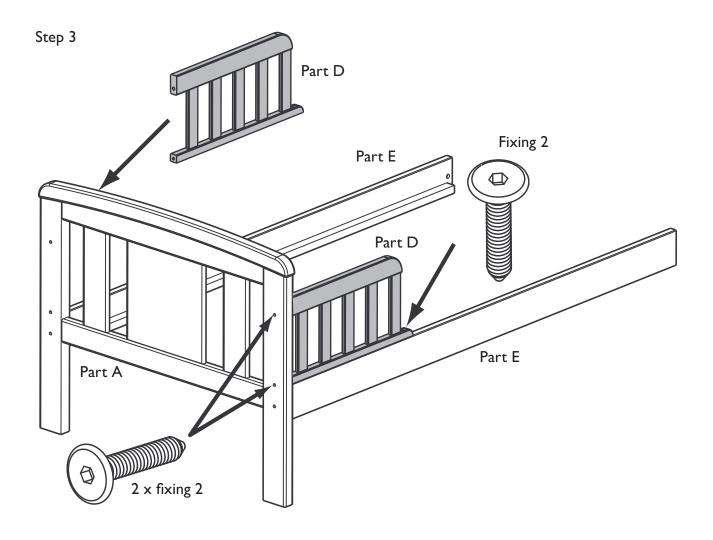
To complete assembly, fit the side rails (part D) to the headboard (part A) and base sides (part E) of the bed. Secure each side rail with three short bolts (fixing 2) as shown.
