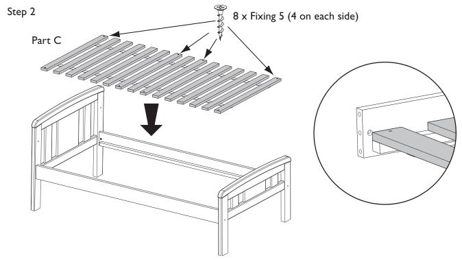
Lay the base slats (part E) on the ledge on the inside of the base sides so that the end slat is level with the end of the ledge as shown. Secure this slat to the base sides using two of the base screws (fixing 5). Move the other end slat toward the footboard as far as the fabric straps will allow and secure this with two more base screws (fixing 5). Finally, secure the two centre slats using four base screws (fixing 5). Once the base slats have been fitted, they should not be removed.
