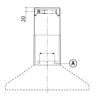
2 Fix the cooker hood to the wall and align it horizontally.
