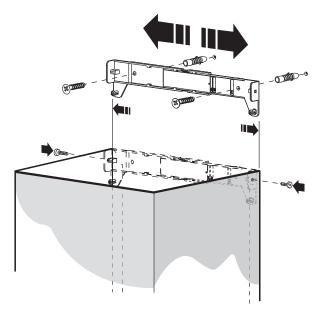
4 Connect the flange (C) to the air exhaust hole.
