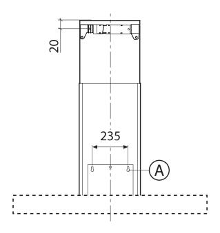
2 Fix the cooker hood to the wall and align it horizontally.
