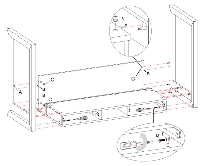
Secure the legs to the top section using screw (D), washer (E) and spring washer (F).
