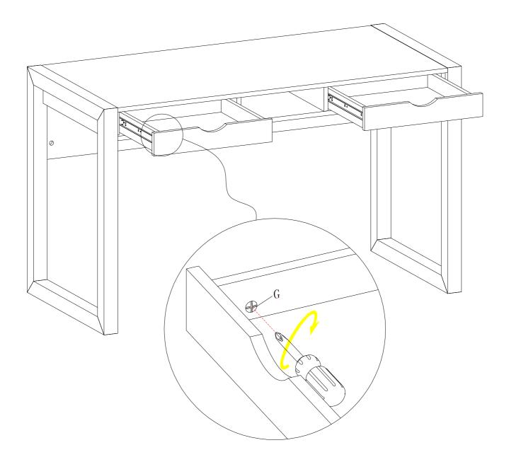
Slide the 2 drawers back into the top section securing the runners with the supplied screw (G). Please do not overturn the screws.
