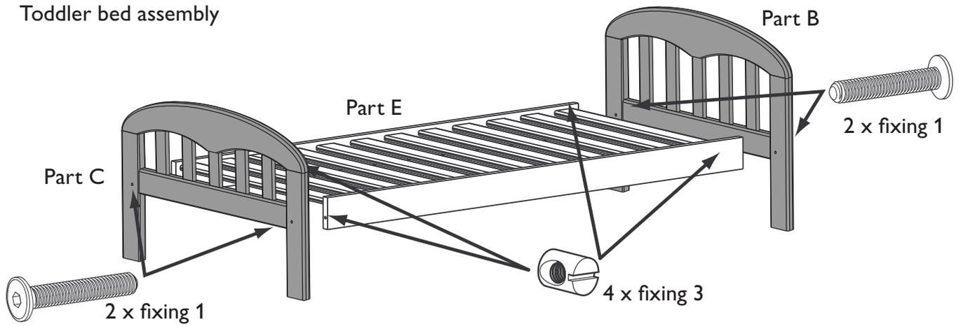
To assemble as a toddler bed, insert four 13mm barrel nuts (fixing 3) into the holes at each corner of the base (part E). Make sure that the slots are visible and, if necessary, use a flat-headed screwdriver to ensure that the slots point towards the holes in the ends. Attach the headboard (part B) and footboard (part C) using four 65mm bolts (fixing 1).
