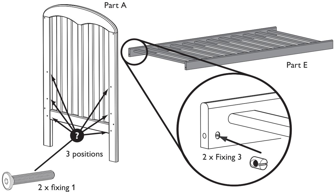
Push two 13mm barrel nuts (fixing 3) into the holes in the base (part E) as shown above. Make sure that the slots are visible and, if necessary, use a flat-headed screwdriver to ensure that the slots point towards the holes in the ends as shown. Select one of the 3 base heights and attach the cot end using two 65mm bolts (fixing 1).
